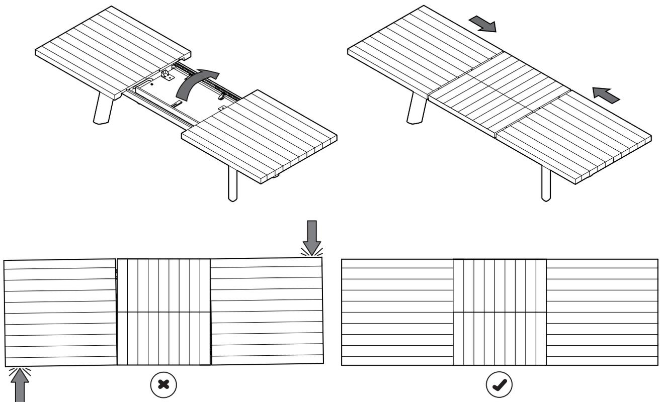
Completely open table, push ends inward and hold whilst second person tightens bolt completely
